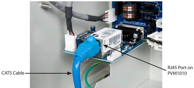
Figure 1-9 Connecting the CAT5 cable to the PVM1010's RJ45 port
