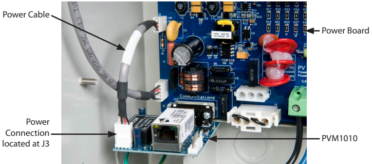
Figure 1-7 Plugging the power cable to the PVM1010's J3 slot
