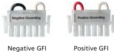
Figure B-8 Negative and Positive GFI Jumpers
