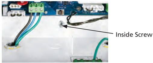
Figure 3-3 Inverter's Inside Screw Below the Power Board
