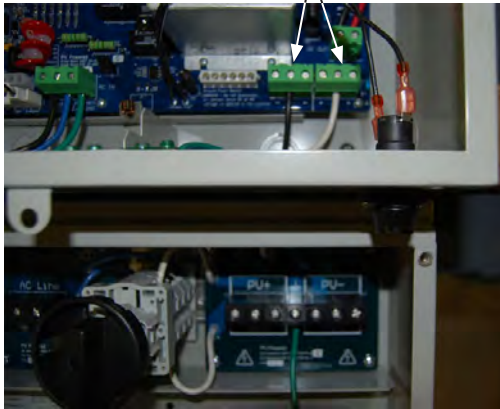
Figure B-1 Inverter's Power Board Terminals
