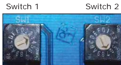
Figure 10: Rotary switches for setting the inverter number on the PVP75kW/PVP100kW
