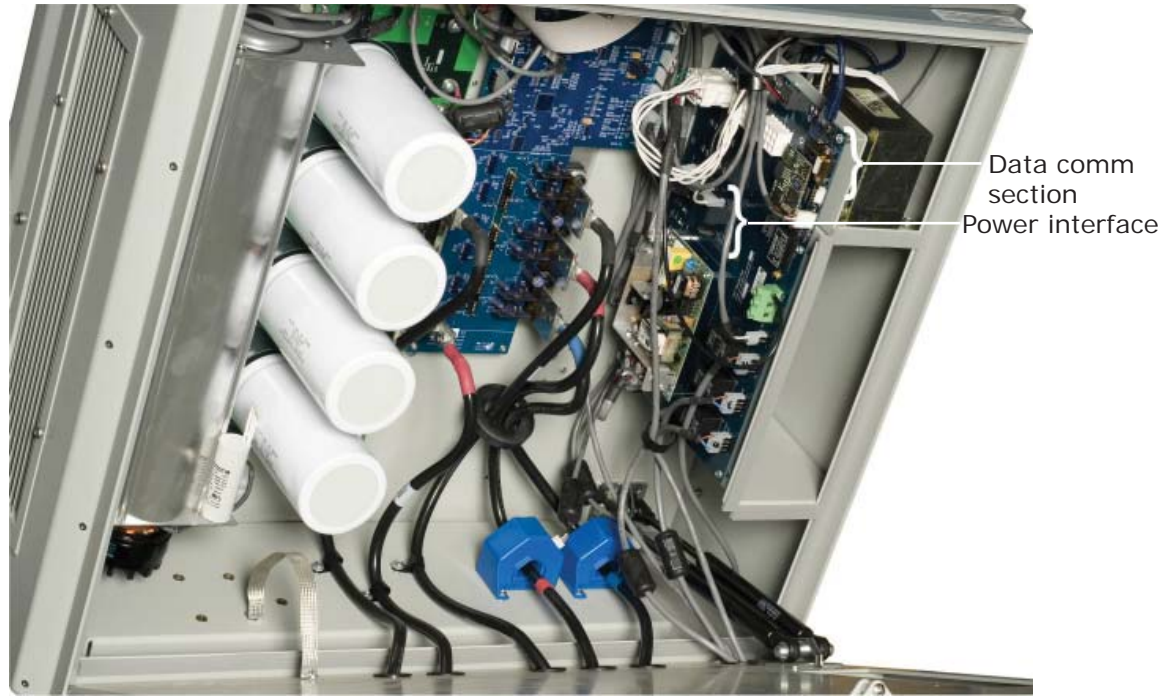
Figure 1: Power interface and data comm sections on PVP30kW inverter
